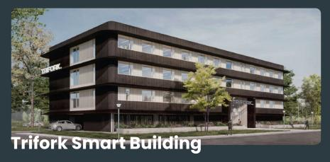
Trifork has set out on a journey to build the ultimate sustainable office building with a minimal climate footprint and an optimal indoor climate and working environment. The building, named Trifork Smart Building One (TSBOne), of approx. 3,000m2 located in Aarhus, Denmark will be made of wood and only a minimum use of concrete and steel.
